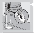
8 Press down the hot water lever and the ambient water lever and let all the water in the clean water tank and in the boiler flow into the container.
