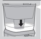
Do not switch on the appliance with the power-on button at the back before the boiler inside the water dispenser is completely filled with water, i.e. when you see water being stored in the clean water tank.
