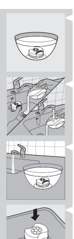
6 Put the Soft water booster in the bowl with the water/salt solution for at least 1 hour. Make sure the Soft water booster is completely submerged.
