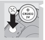
2 Put the 3-volt CR2032 Lithium battery supplied in the battery compartment. You find this battery in the accessory bag.
