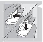
Unlock the child lock. To do so, push the child lock inwards and, at the same time, press down the hot water lever.
