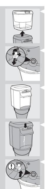
2 Remove the raw water tank and the clean water tank from the appliance.
