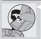
1 Remove the battery compartment cover on the inside of the top cover with a coin.
