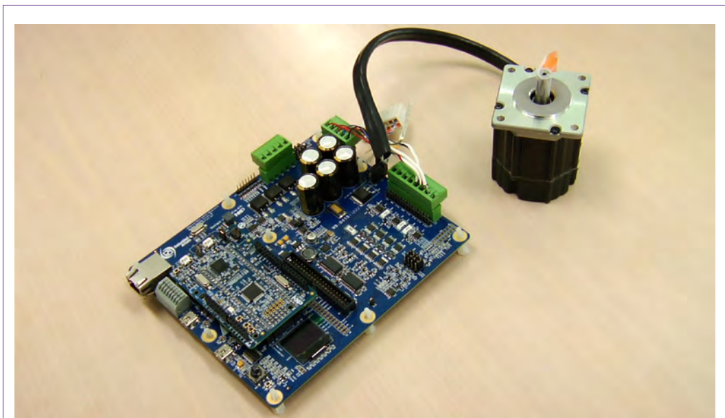
Fig 22. PMSM motor control demo setup
