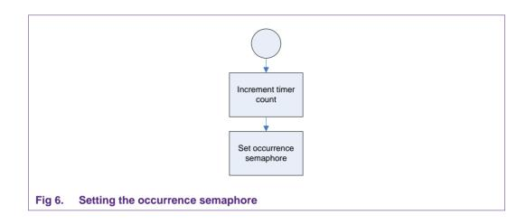
The RTC function also sets an occurrence semaphore, to be tested from the main function. Then it checks the timer counter variable to be within the estimated boundaries. The result of this check is stored into a result semaphore.
