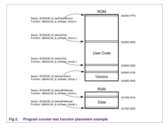
The allocation of the PC dummy test functions are placed accordingly by use of sections defined in the linker file.
