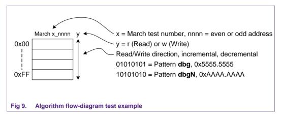
This algorithm is designed to cover both stuck-at faults and direct coupling faults in the fastest possible way.
