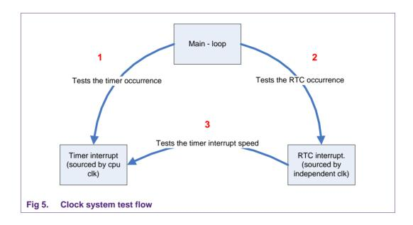
The second function is intended to be called from a timer interrupt service handler. This Timer needs to have the same clock source as the CPU.
