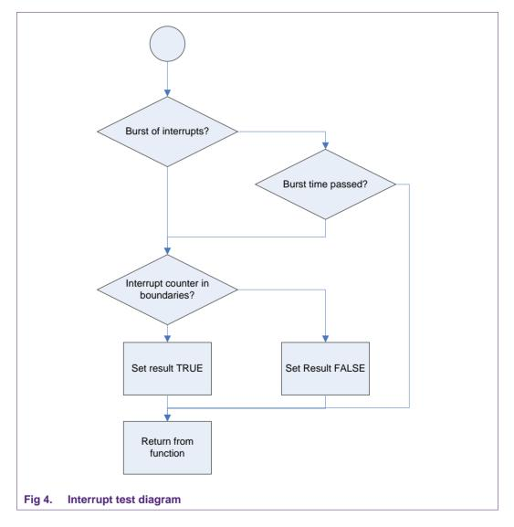
The interrupt check routine first checks the interrupt configuration for the type of interrupt. The test usage details are described in <u>chapter 4.4.2</u>
