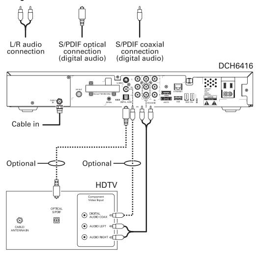
Note: Only (1) HDTV video connection needs to be made to an HDTV.
