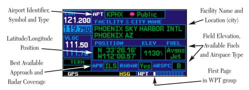
The *airport location page* displays the latitude, longitude, and elevation of the selected airport. The *airport location page* also displays facility name and location, as well as fuel availability, available approaches, radar coverage and airspace type. The following descriptions and abbreviations are used:
