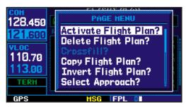
Select "Activate Flight Plan?" from the page menu to begin using the new flight plan. Once the flight plan is created, it may be activated from an options window. Activating the flight plan will place it into "flight plan 00" (a copy of it will still reside in the original catalog location) and replaces any flight plan which currently exists in "flight plan 00."
