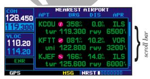
Whenever the GNS 430 is displaying a list of information that is too long for the display screen, a scroll bar will appear along the right-hand side of the display. The scroll bar graphically indicates the number of additional items available within the selected category.
