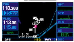
Tuning cursor in the COM window. Use the small ( a) and large ( b) left knobs to dial in the desired standby frequency.
