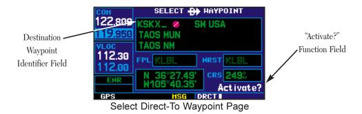
The GNS 430 can use direct point-to-point navigation to guide you from takeoff to touchdown, even in the IFR environment. Once a destination is selected, the unit will provide speed, course and distance data based upon a direct course from your present position to your destination. A destination can be selected from any page with the (direct-to) key.
