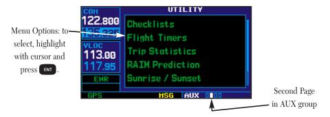
The *utility page* provides access (via "menu options") to checklists, a count down/up timer, trip timers, trip statistics, RAIM (Receiver Autonomous Integrity Monitoring) prediction, sunrise/sunset time calculations and software/database version information. When a menu option is selected, the corresponding page will appear providing additional information and features.
