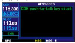
A "COM push-to-talk key stuck" message appears to warn you of a stuck microphone. Transmitting is disabled after 35 seconds of continuous broadcasting.
