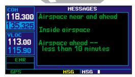
When an airspace alert occurs, the message (MSG) annunciator will flash. Press to view the alert message.
