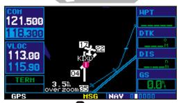
Press and hold the (flip-flop) key for two seconds to activate the 121.500 MHz emergency frequency.
