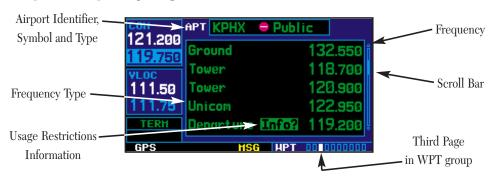
The *airport frequency page* displays radio frequencies and frequency types for the selected airport, as well as sector and altitude restrictions (where applicable). If the selected airport has a localizer-based approach, the localizer frequency(s) is also listed on the *airport frequency page*. The *airport frequency page* may be used to quickly select and tune a COM or VLOC frequency.
