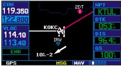
The QLP key allows you to quickly declutter the map display, providing four levels of map detail. Note the "-1" and "-2" ("-3" is also provided) suffix designations above, indicating each successive declutter level.
