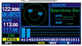
The satellite status page shows the ID numbers for the satellites and the relative signal strength of each satellite received (as a "bar graph" reading.
