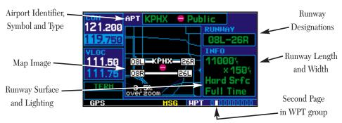
The *airport runway page* displays runway designations, length, surface type and lighting for the selected airport. A map image of the runway layout and surrounding area is also displayed on the *airport runway page*. The map image scale appears in the lower left corner and is adjustable using the Rev. For airports with multiple runways, information for each runway is available.
