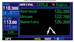
The bottom right corner of the screen indicates which page group is currently being displayed (e.g., NAV or NRST), the number of screens available within that group (indicated by square icons) and the placement of the current screen within that group (indicated by a highlighted square icon). To select a different page within the group, rotate the small right knob ().
