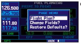
The "Flight Plan?" option allows you to select the numbered flight plan for fuel planning. The "Change Fields?" option allows you to select fuel information for each field as desired.
