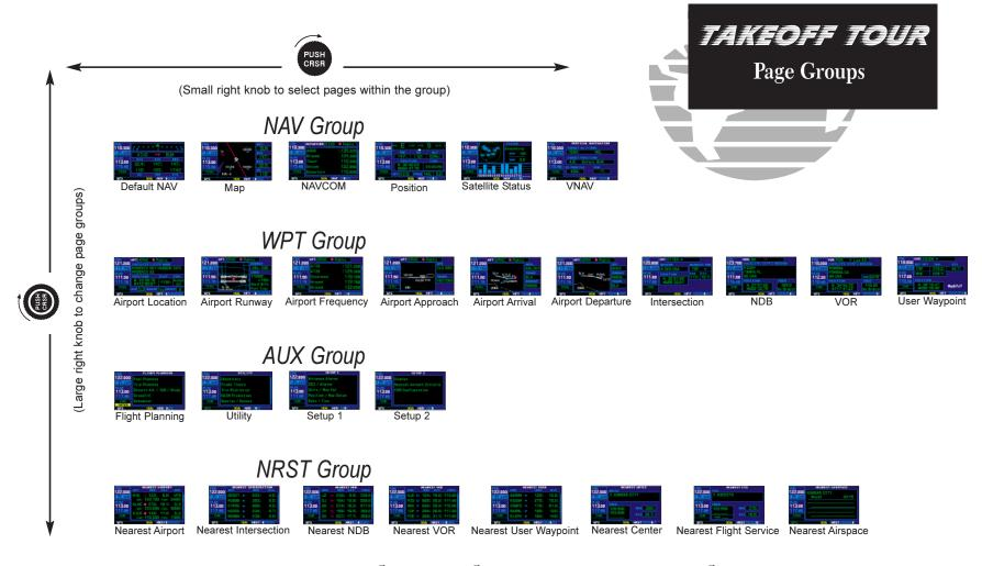
Selection of any main page is performed using the large (ⓐ) and small (ⓐ) right knobs. The large right knob (ⓐ) selects the page group: NAV, WPT, AUX or NRST. The small right knob (ⓐ) selects the desired page within a group. To quickly select the default NAV page, press and hold •••
