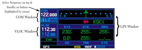
Pushing the small left knob ( ) activates the tuning cursor in the desired frequency window. To select the active frequency, you must first enter the frequency in the standby field, and use the (or ) key to move it to the active field.
