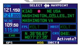
To select the direct-to destination by facility name (shown above) or city location (shown below), highlight the second or third line on the direct-to waypoint page. Use the small (a) and large (b) right knobs to enter the facility name or city. The identifier(s) for any matching entries will appear on the top line of the page.
