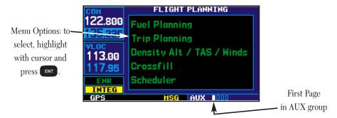
The *flight planning page* provides access (via "menu options") to E6B functions for fuel planning, trip planning, density altitude/true airspeed/winds aloft calculations and a "Crossfill" function to transfer flight plans/user waypoints to a second GNS 430. When a menu option is selected, the corresponding page will appear providing additional information and features.
