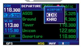
The navigation/communications (NAVCOM) page provides a complete list of airport frequencies at your departure, en route and arrival airports. To place a frequency from this list on standby, highlight the desired frequency and press .
