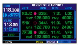
To scroll through the list, press the small right knob (a), then rotate the large right knob (a).
