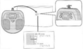
the wood screw into a thick and hard part of the wall, looving 0 -11mm ("/v"-"/v") of the screw projecting from the wall surface. The wall or pillar should be capable of supporting a weight of 5 kg (11 lbs.).
