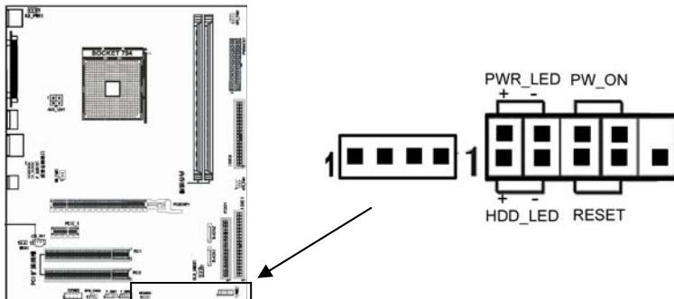
**硬盘动作中指示灯 HDD\_LED (Hard Driver LED Header)**
