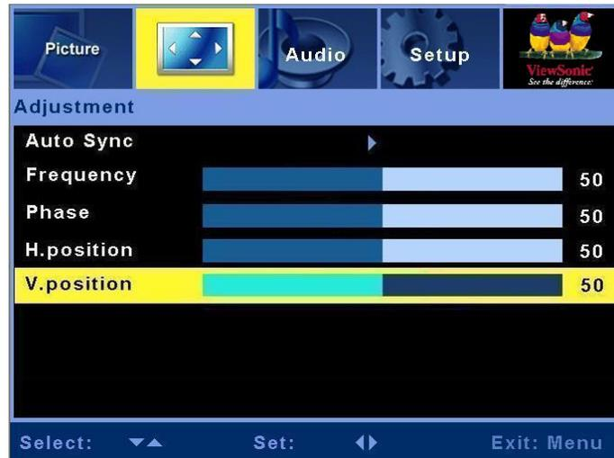
You are most likely to need the adjust menu when configuring the LCD TV for use with PC or S-Video input.
