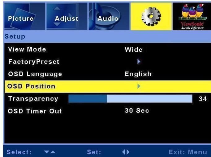
Use this screen to configure the OSD menu and adjust the picture display ratio.
