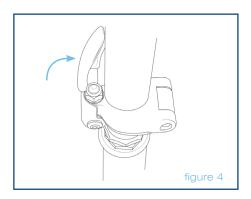
Insert seat post into seat receptacle on frame. Set to desired height and secure in place by inserting thumb screw and turning clockwise until tight.
