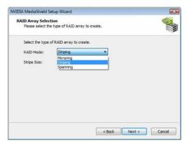
Then, select the type of RAID array to create. You need to choose the RAID Mode first and click Next. Here we take Striping (RAID 0) for example to show you how to use Storage to create Striping (RAID 0). If you plan to use Storage to create other RAID arrays, the operation procedures are similar to the steps of creating Striping (RAID 0).
