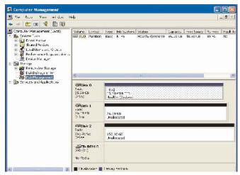
E. The 153.38 GB is for the two disk striped array that was created earlier. To create a partition on it, right click on the Unallocated partition and select New Partition.
