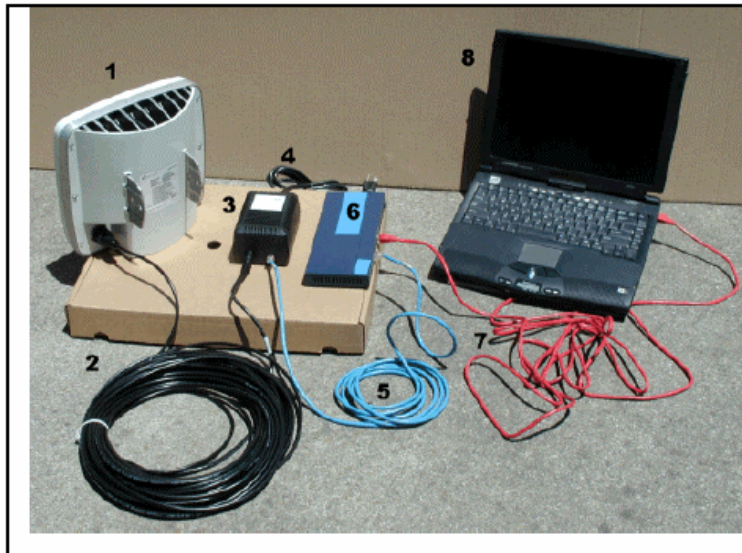
Figure 9. Cable Connections Using a 10/100 Base-T Switch
