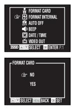
In the set up menu, select "Format Internal" and then press "OK".
