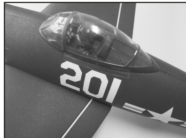
41. Apply instrument panel decal first next trim canopy then secure the canopy in place with furnished decal.
