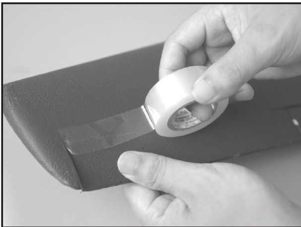
14. Bend the aileron down and apply tape (3/4" wide suggested) on hinge line as indicated. You may rub the hinge, area back and forth with a piece of cloth, this is to smooth the area and increase the tap adhesion.
