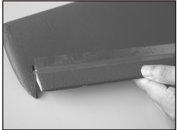
16. Carefully flapping aileron and make sure it move freely but will not come off and tape is sticky enough to hold the aileron in plane.
