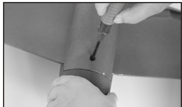
18. Trail fit main wing on fuselage then temporarily secure with M4 washer and wing bolt.
