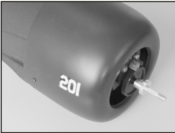
36. Refer to the photo on box top and apply fuselage decal. Trim cowling along with the molded line. Note the orientation of the cowling. Secure the cowling with two 2x8mm washer screws at the molded point.
