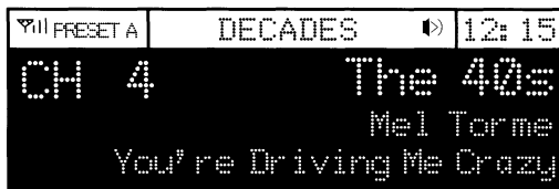
Figure 63. Channel Entry Into a Preset Bank Display
