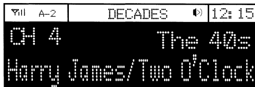
Figure 68. Channel Number and Name Plus Scrolling Artist and Song Title in Large Font
