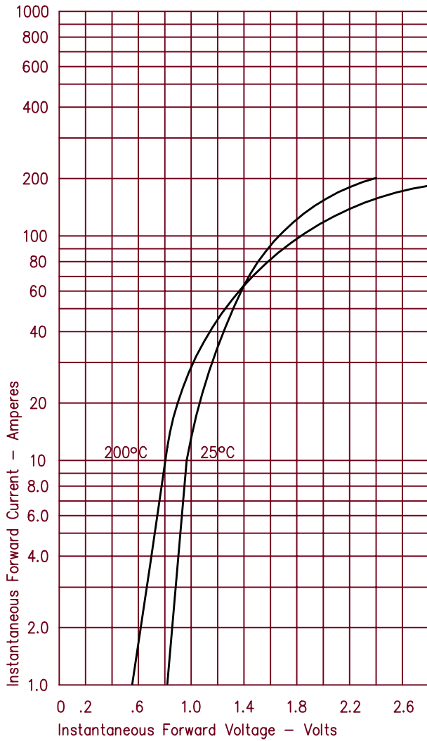
Figure 1 Typical Forward Characteristics – Per Leg
