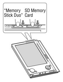
Remove the memory card squarely from the "Memory Stick Duo" slot or the SD Memory Card slot.
