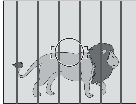
❷ Two or more objects overlapping at different distances within the focus frame (animals in cages, etc.)
