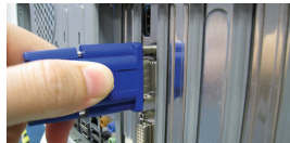
Connect a D-Sub monitor
