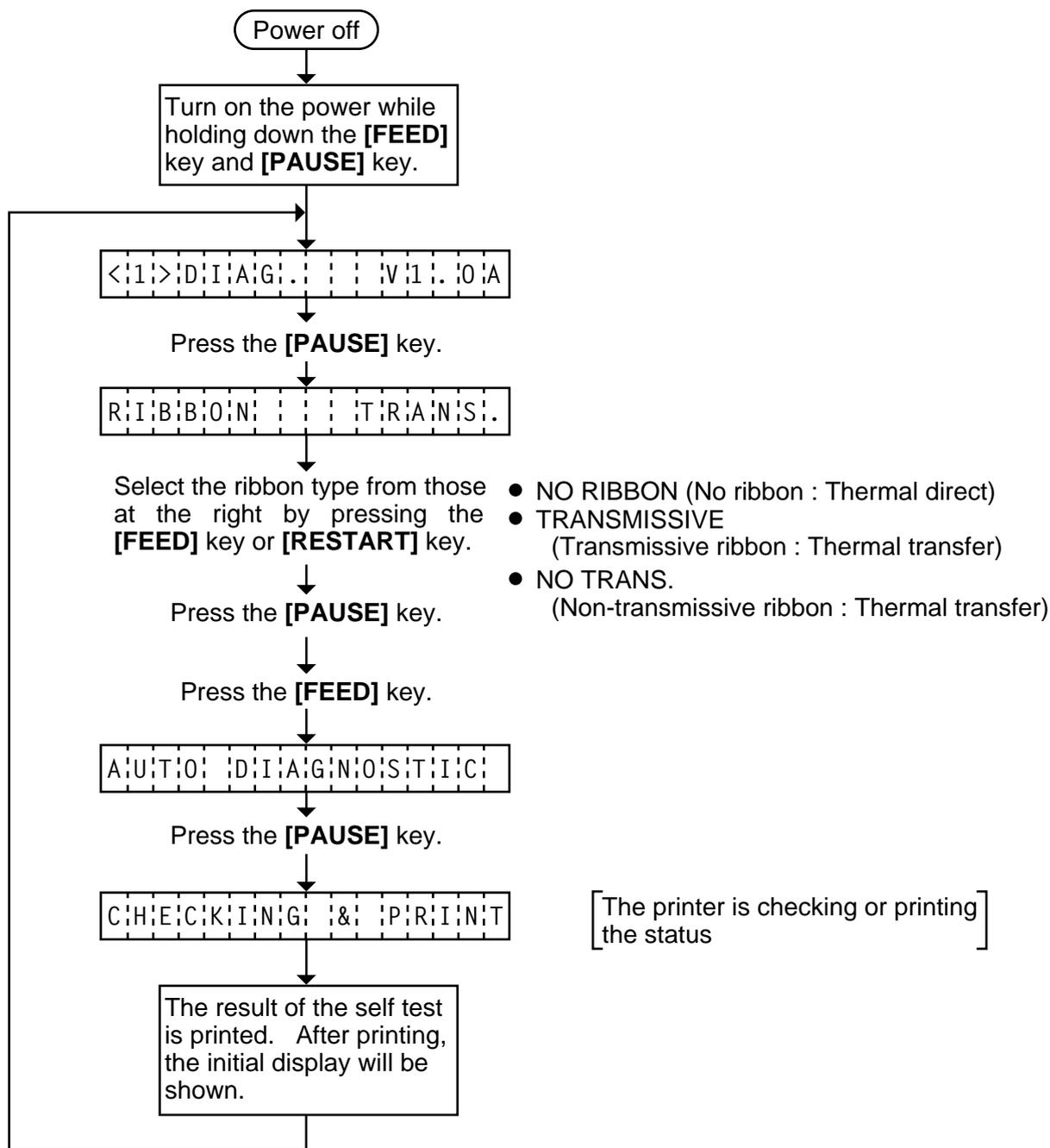
**NOTES:** 1. If the automatic diagnosis printing results in an error, the printer will display the error message and stop printing. The error status can be cleared by the [PAUSE] key, however, the display will return to the initial display "<1>DIAG. V1.0A". Printing is not automatically resumed.
