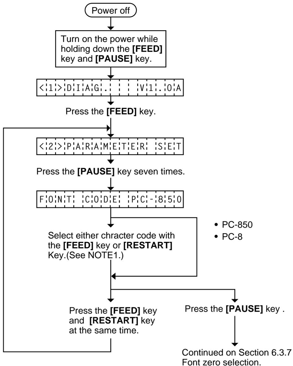
**NOTES:** 1. Holding the **[FEED]** key or **[RESTART]** key down for more than 0.5 seconds enables a fast forward.
