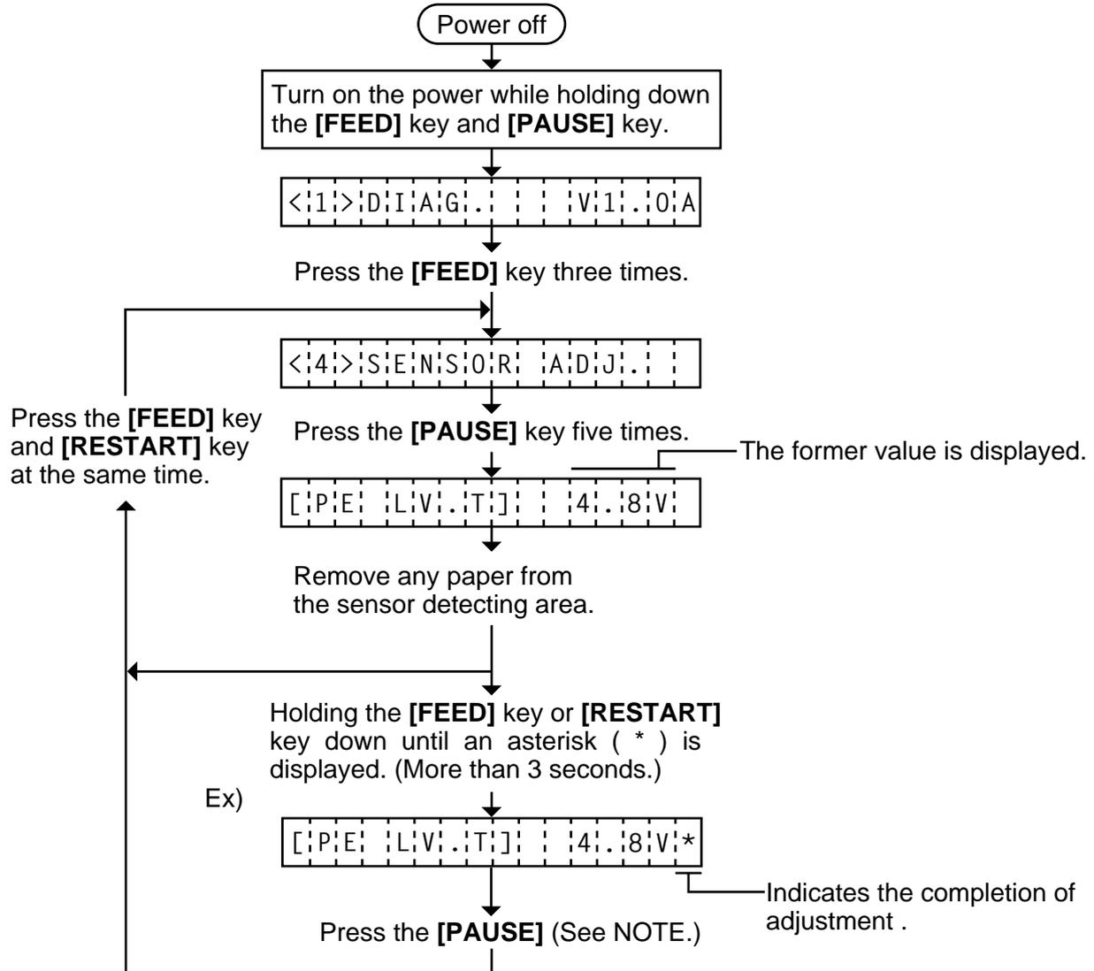
**NOTE:** Pressing the **[PAUSE]** key validates the sensor adjustment. The value of the sensor is displayed up to 5.0 V.
