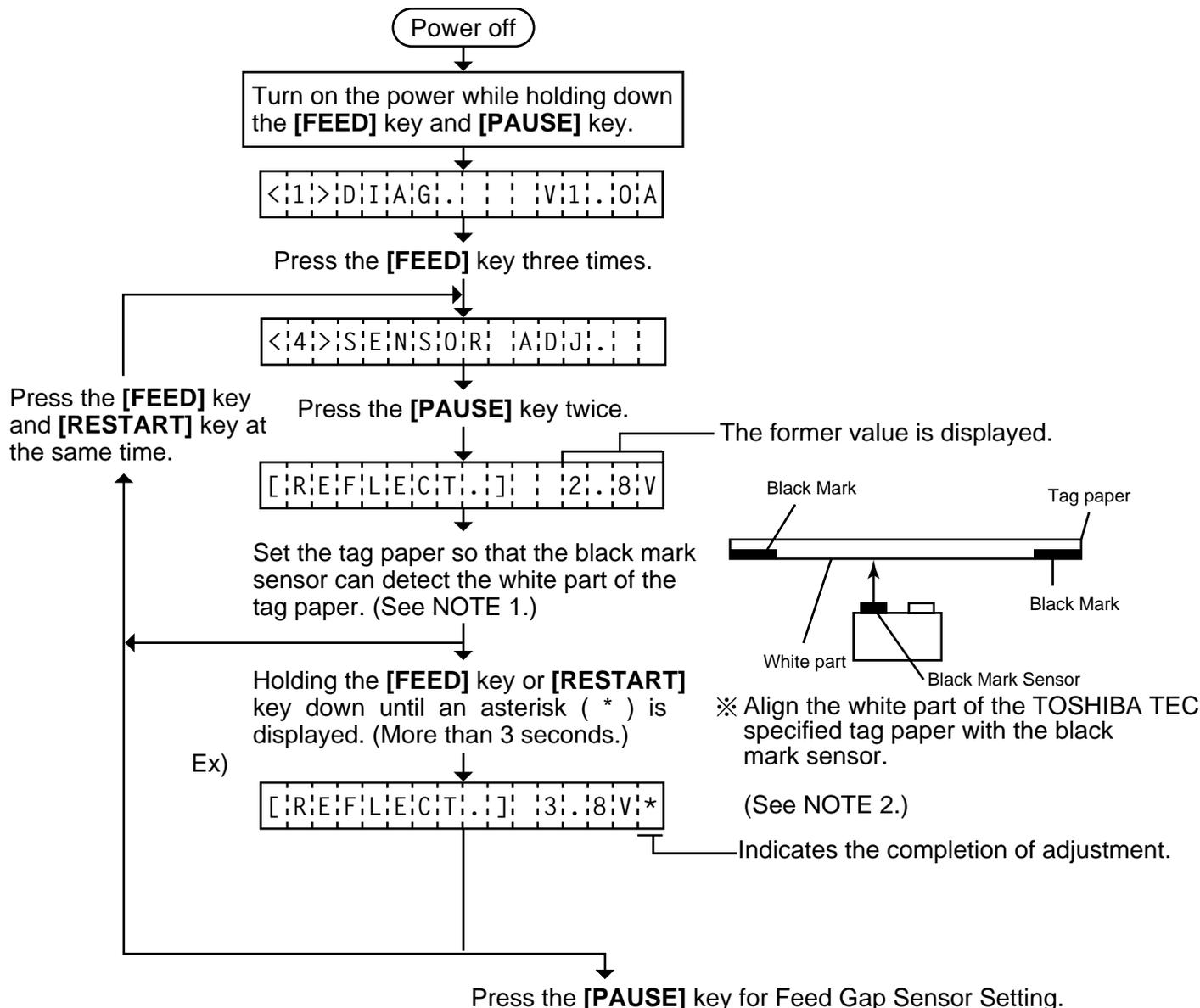
**NOTES:** 1. Make sure to adjust the black mark sensor using the white part of the tag paper as a criterion. Though an adjustment can be performed with the black mark, it may cause a paper jam error.
