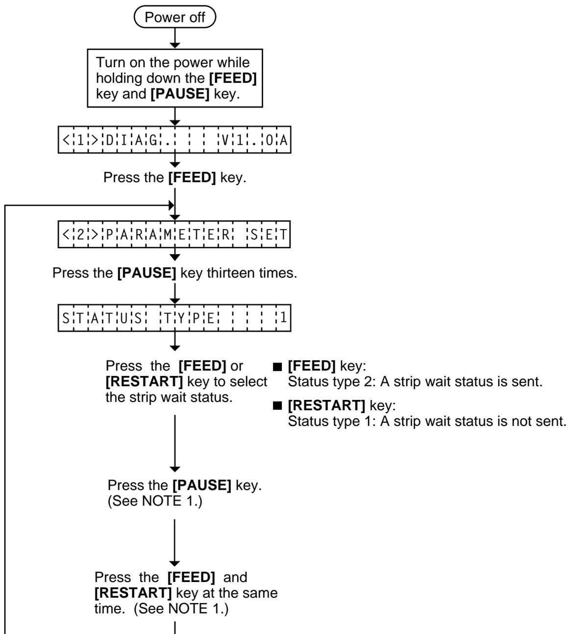
**NOTE:** When the status type 1 is selected, the printer will send (00H) in response to the status request command sent from the PC while a label stays at the strip sensor (when idling, after feeding, or all printing finished).
