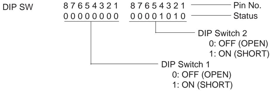
**NOTE:** The DIP switch 1-7 is to be set to 0 (OFF : OPEN) regardless of setting item.
