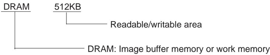
**NOTE:** 1. If an error is detected during DRAM check, the display of readable/writable area will stop when the error occurs.
