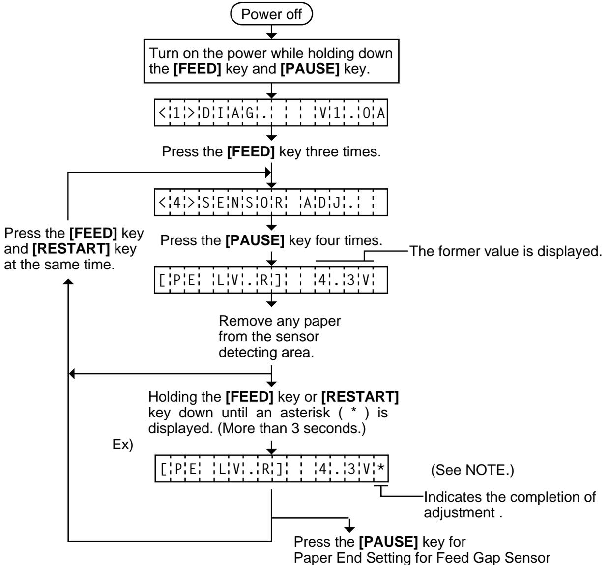
**NOTE:** Pressing the **[PAUSE]** key validates the sensor adjustment. The value of the sensor is displayed up to 5.0 V.
