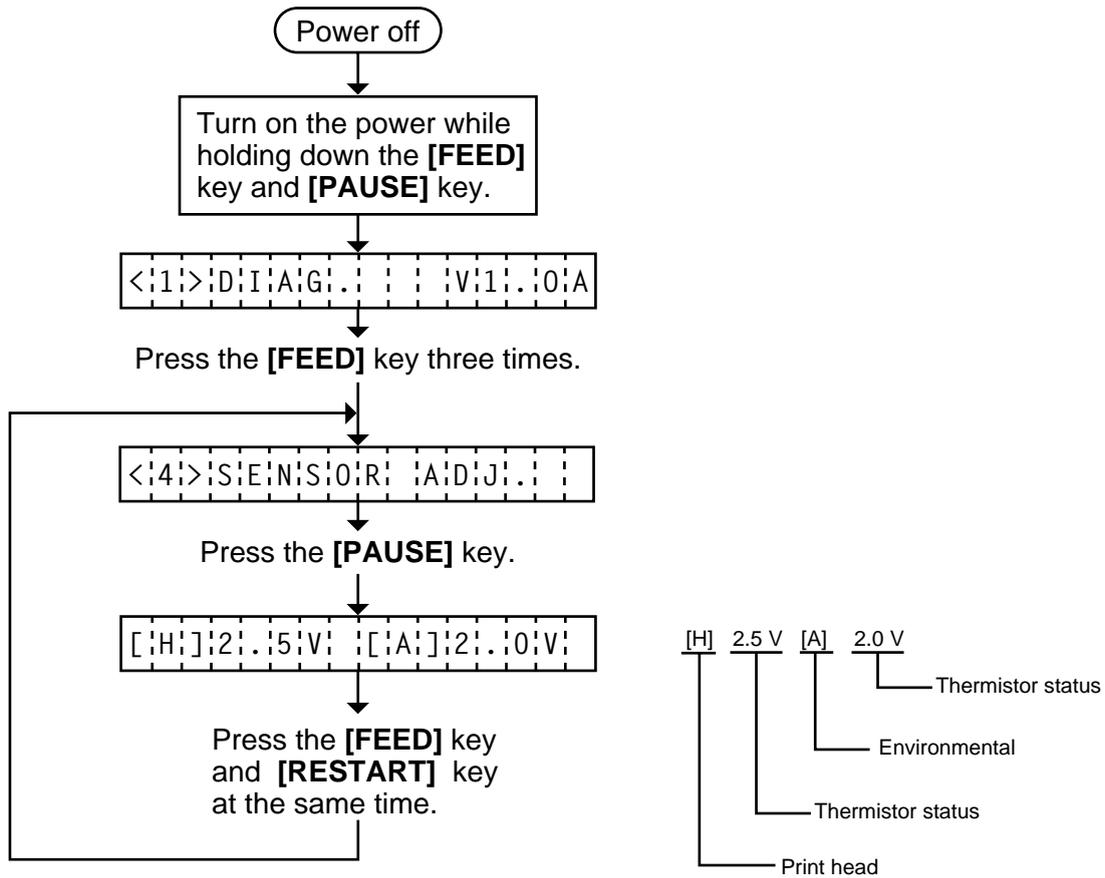
**NOTE:** 1. Since the thermistor is supervised every 200 ms while displaying the status, the display could vary.
