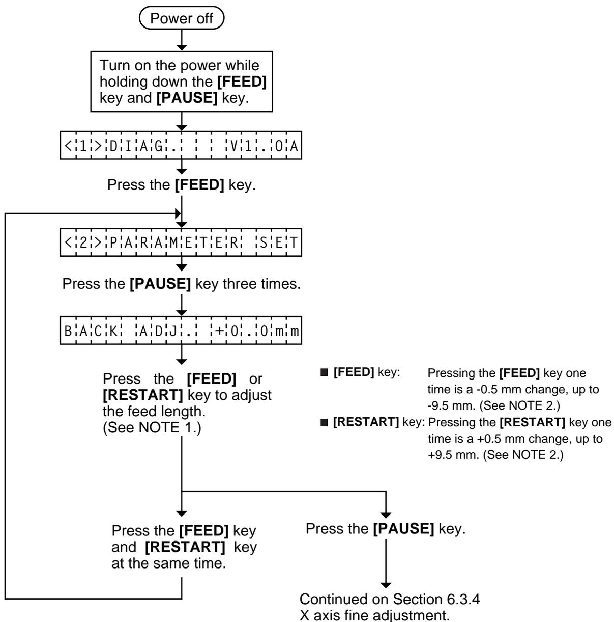
**NOTES:** 1. Holding the **[FEED]** key or **[RESTART]** key down for more than 0.5 seconds enables a fast forward.
