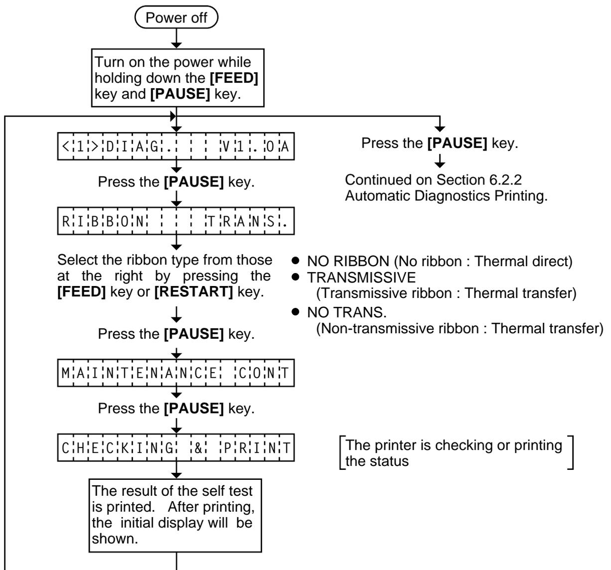
**NOTES:** 1. If the maintenance counter printing results in an error, the printer will display the error message and stop printing. The error status can be cleared by the **[PAUSE]** key, however, the display will return to the initial display "<1> DIAG. V1.0A". Printing is not automatically resumed after the error is cleared.
