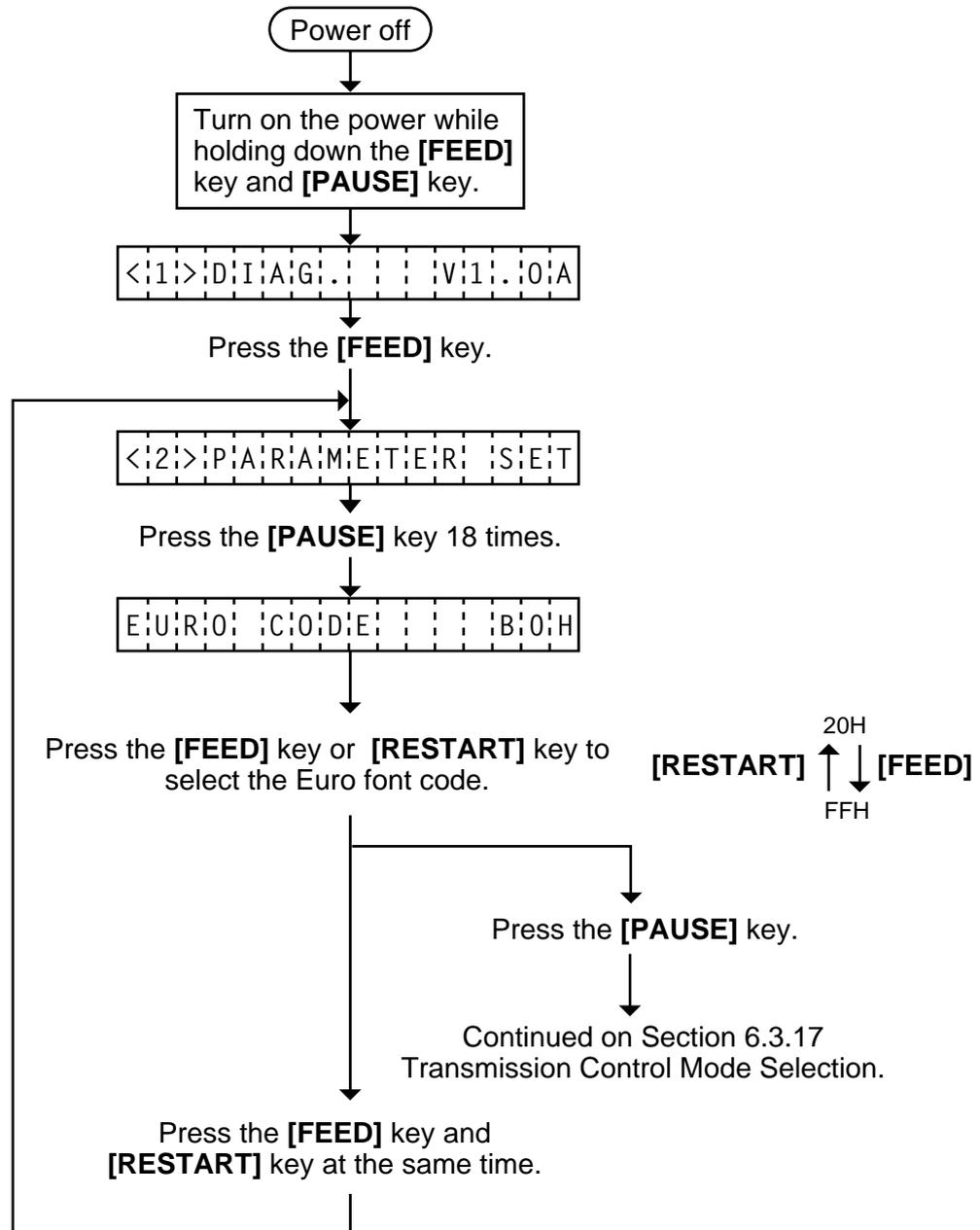
**NOTES:** 1. Holding the [FEED] key or [RESTART] key down for more than 0.5 seconds enables a fast forward.
