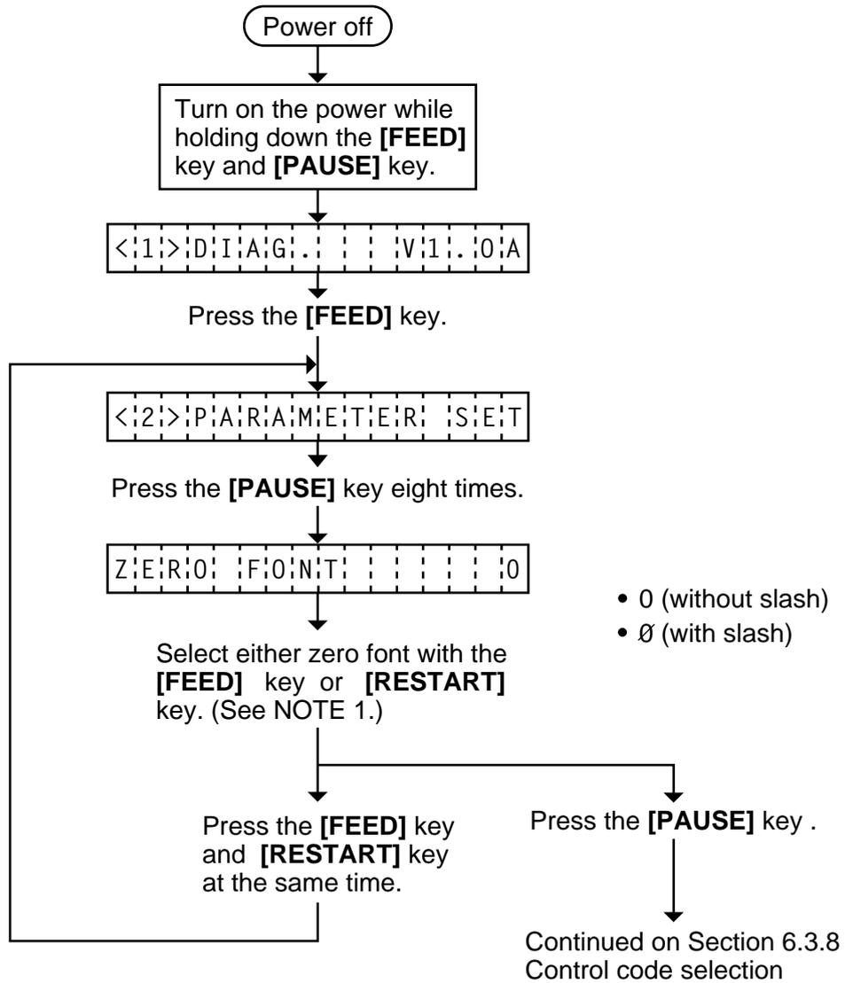
**NOTES:** 1. Holding the **[FEED]** key or **[RESTART]** key down for more than 0.5 seconds enables a fast forward.
