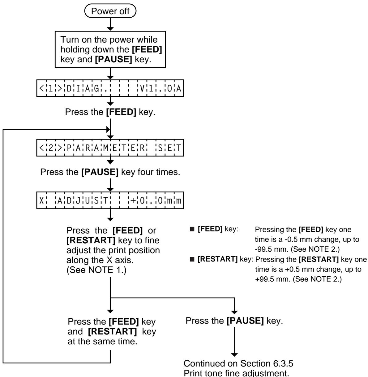
**NOTES:** 1. Holding the **[FEED]** key or **[RESTART]** key down for more than 0.5 seconds enables a fast forward.
