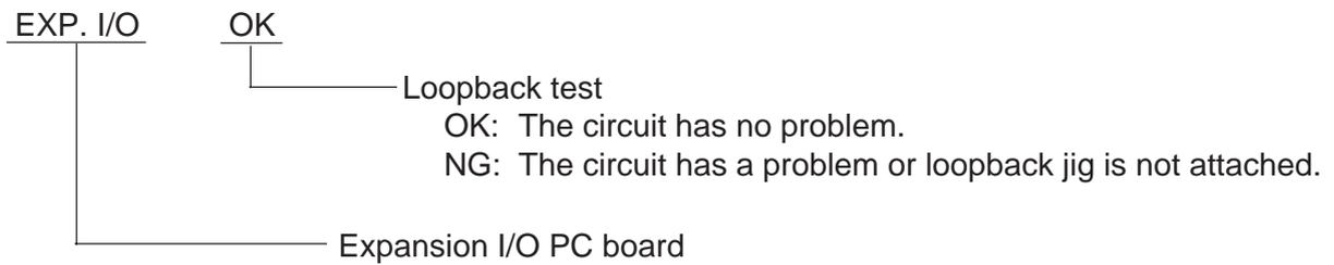
For the loopback test, connect a jig as shown below and check HIGH output / HIGH input and LOW output / LOW input.
