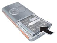
1 Insert the battery with the label side up and the connectors facing each other.
