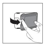
3 Clean the sensor, the dust inlet and outlet with a lightly moistened cotton swab, and finish with a dry cotton swab.
