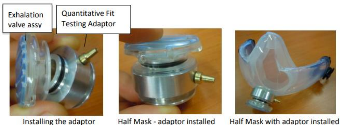
FIGURE 6: INSTALLING THE HALF MASK FIT TEST ADAPTOR (PAF-0025)
