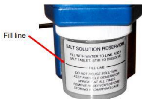
FIGURE 10: PORTACOUNT™ PARTICLE GENERATOR FILL LINE
