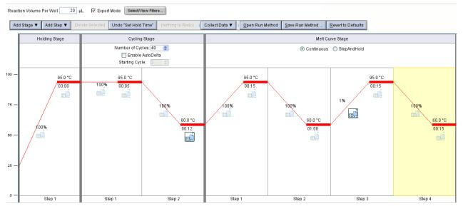
**Note:** If you do not require a high-resolution melt curve, you can select the **StepAndHold** option for the melt curve stage and then increase the ramp rate to 0.5°C per second to shorten the protocol time.
