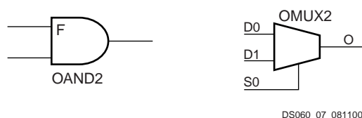
Figure 7: AND and MUX Symbols in Spartan-XL IOB
