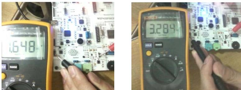
图 3.10.9 实验结果 (左: DAT=0x7FF, Vout=1.65V; 右: DAT=0xFFF, Vout=3.29V)
