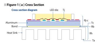
substrate to the grease ( adhesive ). The thermal resistance between the junction section of the light-emitting diode and the aluminum substrate side of the package outer shell is Rj-c, and the specific thermal resistance value of the package. Therefore, the following formula is used
