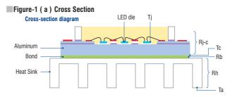
substrate to the grease ( adhesive ). The thermal resistance between the junction section of the light-emitting diode and the aluminum substrate side of the package outer shell is Rj-c, and the specific thermal resistance value of the package. Therefore, the following formula is used
