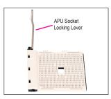
Step 1: Completely lift up the APU socket locking lever.
