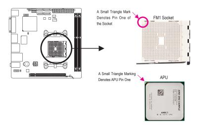
B. Follow the steps below to correctly install the APU into the motherboard APU socket.
