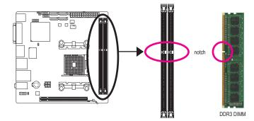
Before installing a memory module, make sure to turn off the computer and unplug the power cord from the power outlet to prevent damage to the memory module.
