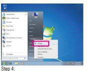
After the operating system is installed, click **Start**, right-click the **Computer** and select **Manage**. Go to **Disk Management** to check disk allocation.
