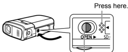
Check that the red marker of the lock is no longer visible.
