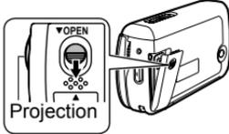
Slide the lock to the OPEN side and lift the projection with a finger to open.
