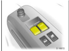
Operational with key in ignition switch position ON.
