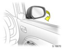
For the safety of pedestrians, the exterior mirrors will swing out of their normal mounting position in the event of an accident-like impact.
