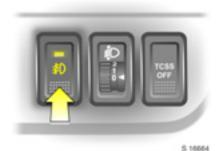
The front fog lamps can only be switched on when the ignition is on and the light switch is in position ● or ■O.
