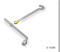
4. Attach the jack handle to the wheel bolt wrench (as shown in illustration) and insert hook end of jack handle through jack eye. Before positioning the jack, set it to the necessary height by rotating the jack handle clockwise using the attached wheel bolt wrench.
