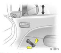
The door windows can be operated with the crank.
