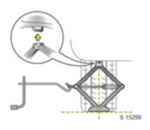
5. Position jack at the front or rear jacking point located nearest to the wheel concerned so that the jack claw spans the vertical base. Make sure it is properly positioned, ensuring the jacking bar fits securely into the jack head groove.
