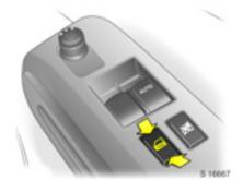
Use the central locking switch to lock or unlock the doors and tailgate from inside the vehicle.
