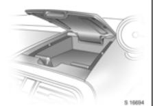
The instrument panel upper tray is located above the centre air vents. To open, lift front edge of lid.
