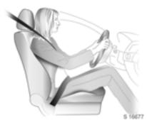
The front and rear seats are equipped with three-point seat belts with automatic retractors and locking devices, allowing freedom of body movement when the vehicle moves at a constant speed, although the spring-tensioned belts are always a snug fit.
