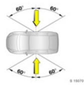
The side airbag system will be triggered depending on the severity of the accident and within the range shown in the illustration.
