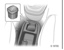
The portable ashtray can be fitted in the front or rear cup holder in the centre console.
