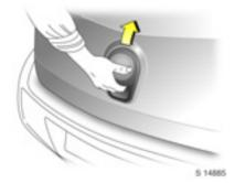
The tailgate can be opened by operating the button below the handle and lifting the tailgate.
