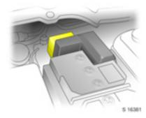
The fusebox is located behind the rear of the battery.
