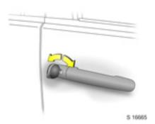
The doors may be manually locked and unlocked using the key.
