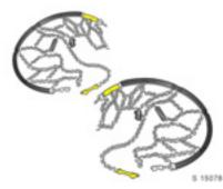
Tyre chains are only permitted on the drive wheels (front axle). They must be fitted to the tyres symmetrically in order to achieve a concentric fit.
