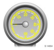
Indicates the engine speed in revolutions per minute (rpm).
