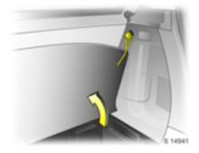
To access the under floor storage, pull up floor carpet using the central strap located near the tailgate latch and hang the string on the hook provided.
