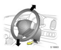
To adjust steering wheel \*, pull lever forwards, adjust height, push lever back and engage.
