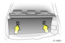
The Top-Tether mountings located on the rear of the seatbacks are designed to hold child restraints which come equipped with a top-tether mounting strap only.
