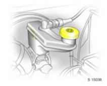
The brake fluid level in the reservoir must not be higher than the **MAX** mark or lower than the **MIN** mark.
