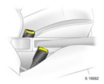
The seat belt systems on the front seats incorporate belt tensioners housed in the belt buckles and seat belt retractors.
