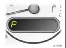
Display of the selected gear or mode with automatic transmission.
