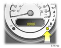
To change brightness level, switch on headlamps and press the **MODE** button repeatedly until the squares that indicate the brightness level appear in the odometer display. Then press and hold the **MODE** button to cycle through brightness levels.
