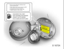
The fuel filler neck is located on the left rear side of the vehicle.
