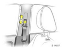
Height adjustment of front seat belt upper anchorage points.
