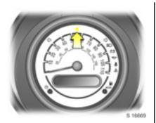
The theft-deterrent control indicator starts flashing after the key is turned to positions LOCK or ACC, or removed from the ignition switch.
