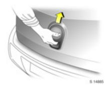
To unlock and open the tailgate: Press button on remote control, operate button below the handle
