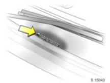
The visible VIN may also be stamped on a plate and affixed to the instrument panel on the driver's side, visible through the windscreen.
