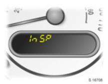
In the case of vehicles with fixed engine oil change and service intervals, **InSP** appears in the odometer display if the ignition is switched on when servicing is
