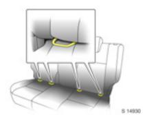
The ISOFIX mountings located between the seatback and seat cushion are used for mounting ISOFIX child restraint systems on the outboard rear seats.
