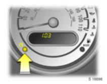
The time is shown in the odometer display when the ignition is switched on.
