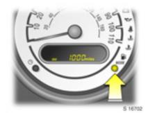
The odometer indicates how far the vehicle has been driven.
