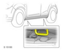
The location of front and rear jacking bars may be indicated by notches on the bottom edge of the vehicle, under the doors.
