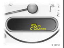
Range is calculated from current fuel tank content and instantaneous consumption. The display shows average values.
