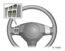
Infotainment system functions can be operated with the buttons mounted on the steering wheel.
