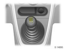
Reverse: with the vehicle stationary, wait 3 seconds after declutching before engaging gear. If the gear does not engage, set the lever in neutral, release the clutch pedal and depress again; then repeat gear selection.
