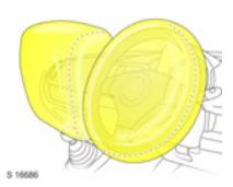
When triggered, the airbags inflate in milliseconds. Forward movement of the driver and front passenger is checked and the risk of injuries to the upper body and head are thereby substantially reduced.
