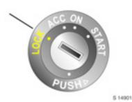
The system checks whether the vehicle may be started using the key that has been inserted. If the key is recognised as "authorised", the vehicle can be started. The check is carried out via a transponder housed in the key.
