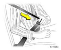
Pull the belt out evenly from the retractor and guide it over the shoulder, making certain that it is not twisted at any point. The belt must not rest against your neck or arm.
