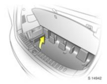
If necessary, the under floor storage compartment can be removed from the luggage compartment.
