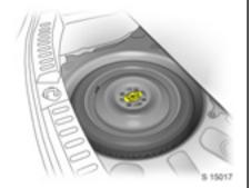
The temporary spare wheel is located in the luggage compartment and is secured with a screw-in retainer.
