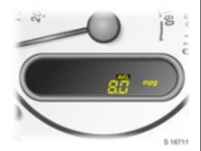
Display of average fuel consumption. The measurement can be restarted at any time.
