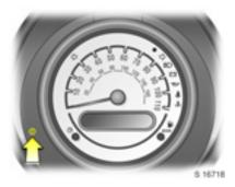
If there is a problem with the automatic transmission, control indicator  $\Phi$  flashes. The transmission no longer shifts automatically.
