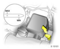
The illustrations show checking the engine oil in the K 10 B and K 12 B petrol engines and the diesel engines respectively.
