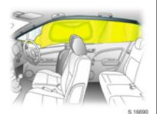
When triggered, the airbags inflate in milliseconds. The risk of injury to the head in the event of a side impact is substantially reduced.
