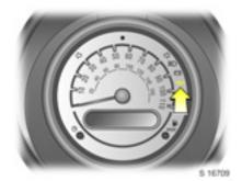
Indicates when the engine oil and oil filter require changing. Based on driving conditions, the interval at which an oil change will be indicated can vary considerably.
