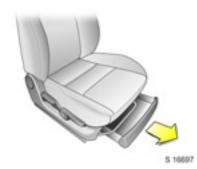
The front passenger's seat has a tray located beneath the seat.
