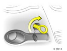
Screw in towing eye attachment clockwise until it is firmly in place. If necessary, use jack handle to tighten.
