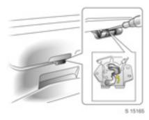
If the central locking system \*cannot be operated with the remote control, the tailgate can be opened from inside the vehicle.
