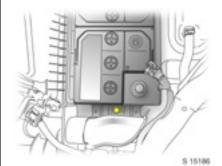
Unscrew the retaining bolt using a suitable tool and remove battery, coolant expansion tank and fuse box.
