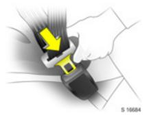
Insert the latch plate into the buckle. Seat belt buckles are designed such that latch plates cannot be inserted in the incorrect buckle. The centre rear seat belt buckle is distinguished by appropriate lettering on the buckle.
