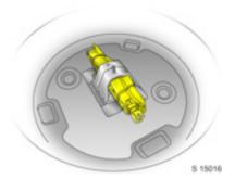
To access the jack and vehicle tools, open tailgate and pull up luggage compartment floor carpet using the central strap located near the tailgate latch and hang the string on the hook provided ♀ 4-4.
