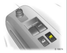
Press the 🗷 switch in driver's door to deactivate front passenger's door electric window operation when a child is occupying the seat.
