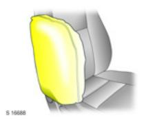
When triggered, the airbags inflate in milliseconds. The risk of injury to the upper body and pelvis in the event of a side impact is thereby substantially reduced.
