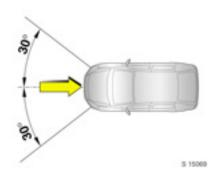
The front airbag system will be triggered depending on the severity of the accident, and within the range shown in the illustration.
