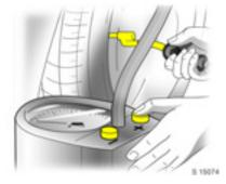
After having checked the tyre pressures, securely tighten the valve caps.
