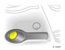
Access the rear of the fog lamp from behind the front bumper.
