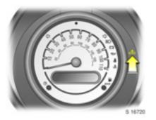
If regeneration of the diesel particle filter is not successful or possible, control indicator & may illuminate and the vehicle goes into limp home mode: interrupt your journey and seek the assistance of a workshop immediately.
