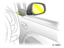
Adjust mirrors by swivelling lever in required direction.
