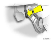
Depress accelerator pedal past the pressure point and hold in position; below certain speeds, the transmission shifts down into a lower gear.
