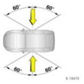
The curtain airbag system will be triggered depending on the severity of the accident and within the range shown in the illustration.
