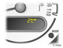
The outside temperature is shown in the odometer display when the ignition is switched on.
