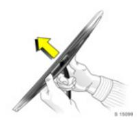
Lift wiper arm. Disengage wiperblade as shown in illustration and remove.
