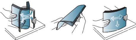
3. After inserting paper into the tray, adjust the support guide so that it lightly touches the paper stack.
