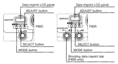
•Adjusting date and time (Example: year 2000, April 21, 15:30; shows the operation with F80D; same operation with F80S) *I* Push MODE button to select one of the date displays.
