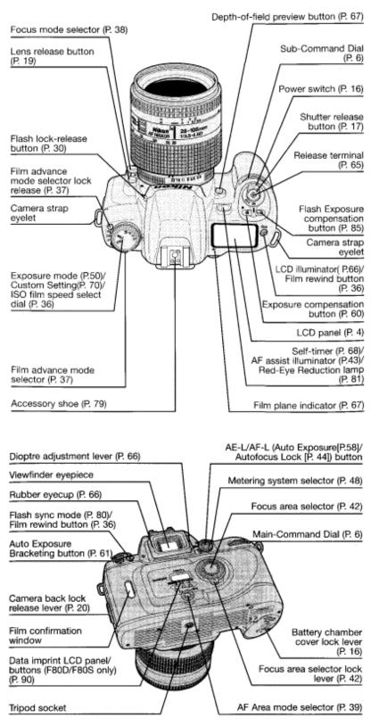
\* Illustration shown is the F80D. The camera backs of the F80 and F80S differ from the F80D. For the F80S's camera back, see page 90.
