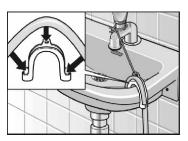
Drainage into a wash basin( The hose elbow is in the drum). **Caution**
