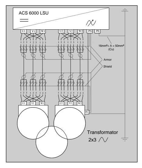
The picture presents a typical installation with three parallel 3-core-cables and an additional grounding cable.
