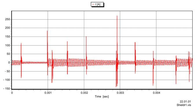
The RMS value of the shield current is about 20A. Current peaks up to 250A are to be expected.
