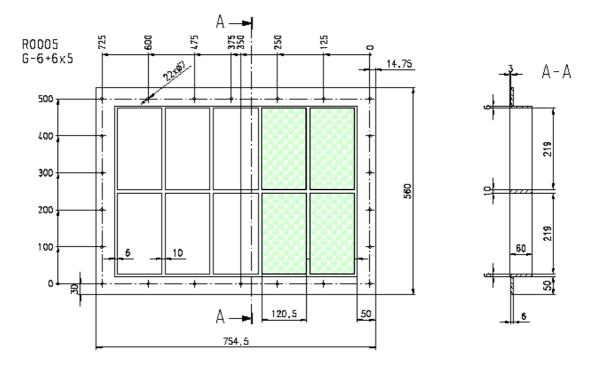
These frames, which are delivered with the drive, can be equiped with different filler modules. The modules have to be provided from the customer. The following table shows the range of available modules:
