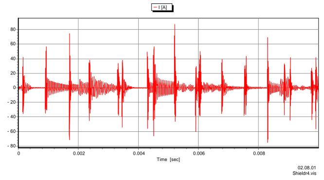
The RMS value of the shield current is about 10A. Current peaks up to 100A are to be expected.
