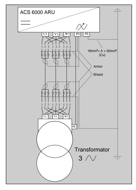
The picture presents a typical installation with three parallel 3-core-cables and an additional grounding cable.
